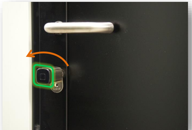
To lock the door, please hold your keycard to the sensor once again and turn the doorknob leftwards.
